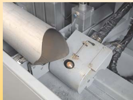
CrNi-tubes (1.4301) with metallic clean and dross-free cutting surface
